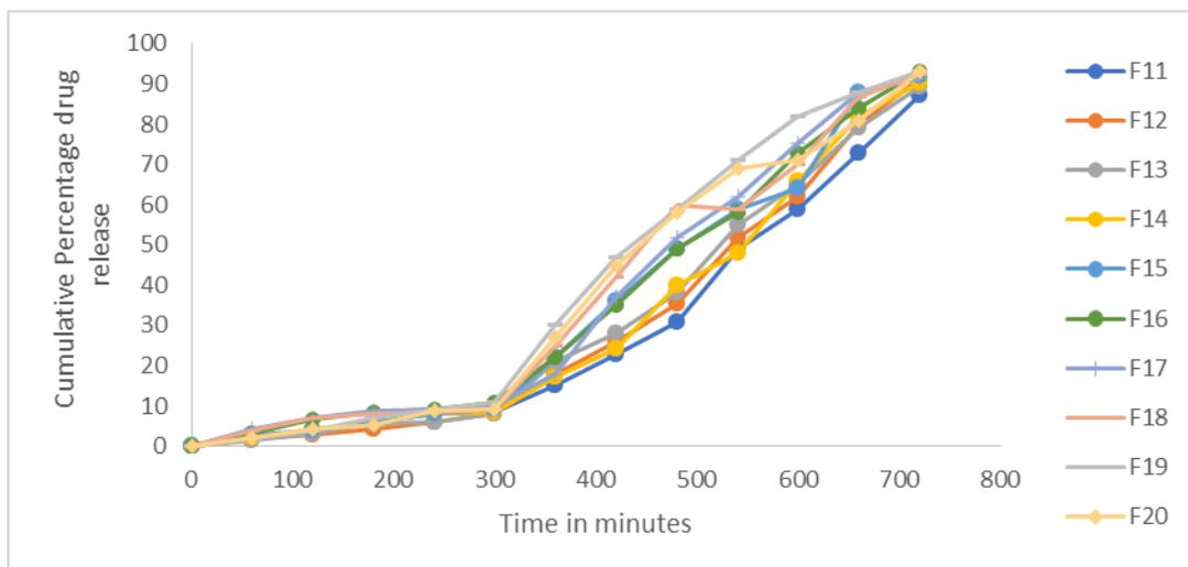
Fig. 6 *In vitro* release profile of etodolac solid dispersions formulations F11-F20
