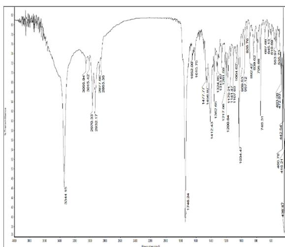
Fig. 1 FTIR spectral data of etodolac
